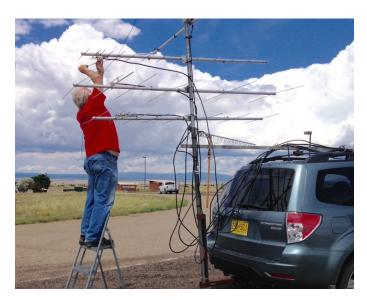
My rover, configured for 50MHz to 2304 MHz is shown above. There is a 24 GHz Gunnplexer in the car. The TS-2000X covers 50, 144, 432 and 1296 Mhz. I use 222 Mhz and 902 Mhz transverters to activate the additional bands. Most contacts are made on SSB or CW but I'm working more contacts lately on FM as well, and they really help. The picture above was taken during the June 2015 VHF/UHF contest in DM74, near the Torrance County landfill; a favorite operating spot near the Moriarty grid convergence.
