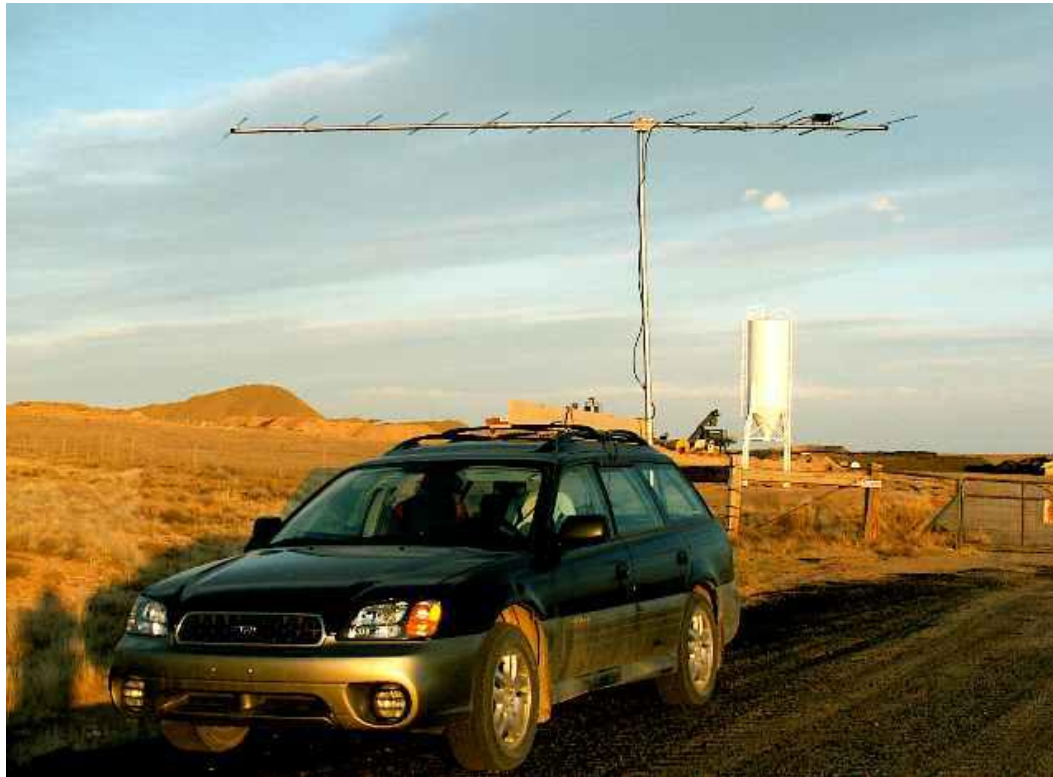
13 element Cushcraft 13B2 set up for 2M sprint in DM74
